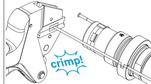
**08** Press both crimp caps into the ring with the front of the YCP-ACT-2 crimping tool
