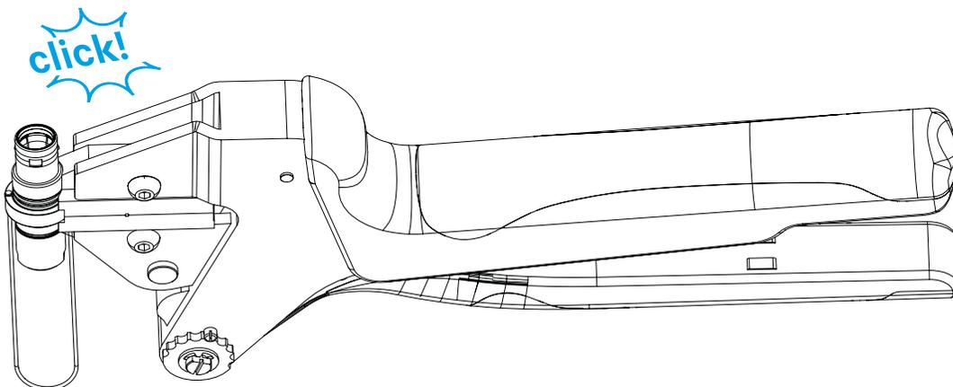
**09** Pull at the unlocking lace for easy release of the connector
