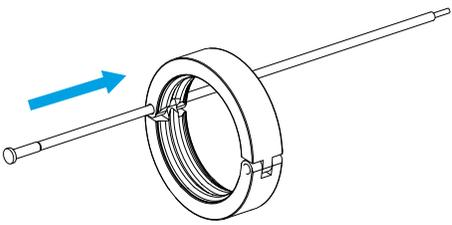
**05** Place half rings around the connector at the height of the waves and close the rings
