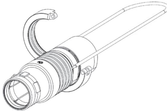
**06** Thread the release tape through the cavity on the other side of the ring and place the end cap on the end
