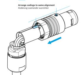
O7 Slide the back side of the elbow part over the dovetail of the first elbow part.
