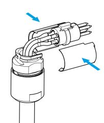
Slide the housing onto the halfshells
