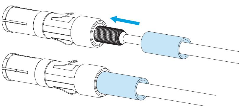
07 Put the crimping ferule into the crimp insert in shaft 2.67mm and Crimp the ferule
