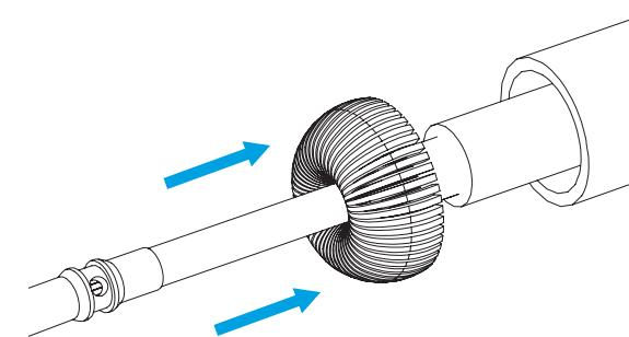
05 Insert the inner contact into the coax contact until You hear a click
