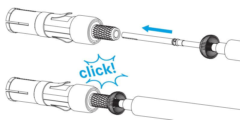
06 Cover the knurled surface with the shielding and push the crimp ferule forward
