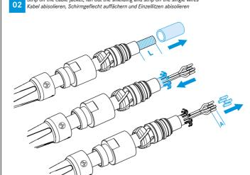
Strip off the cable jacket, fan out the shielding and strip off the single wires
