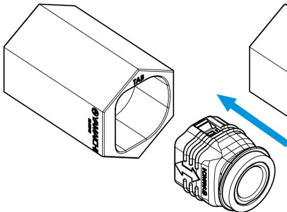
**07** Insert the Plug, cablesealing, plug stopper and the sealscrew into the IP67 cover. Make shure that the TAB on the Plug is in the right position to the TAB-Mark on the Y-CON-TOOL-40
