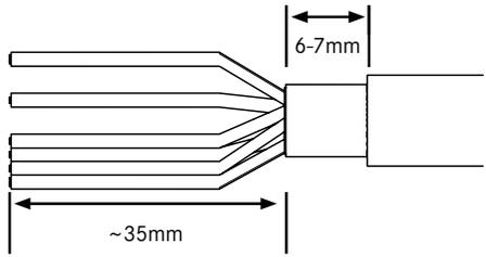
**02** Thread single wires into the insert as shown
