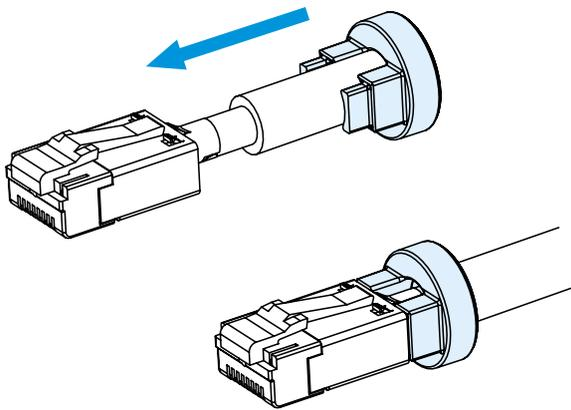
**04** Push the cablesealing to the plug stopper
