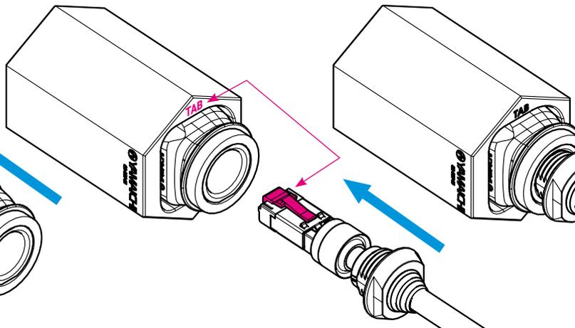
**08** Use a 17mm wrench to turn the sealingscrew into the IP67 cover until machanical stop
