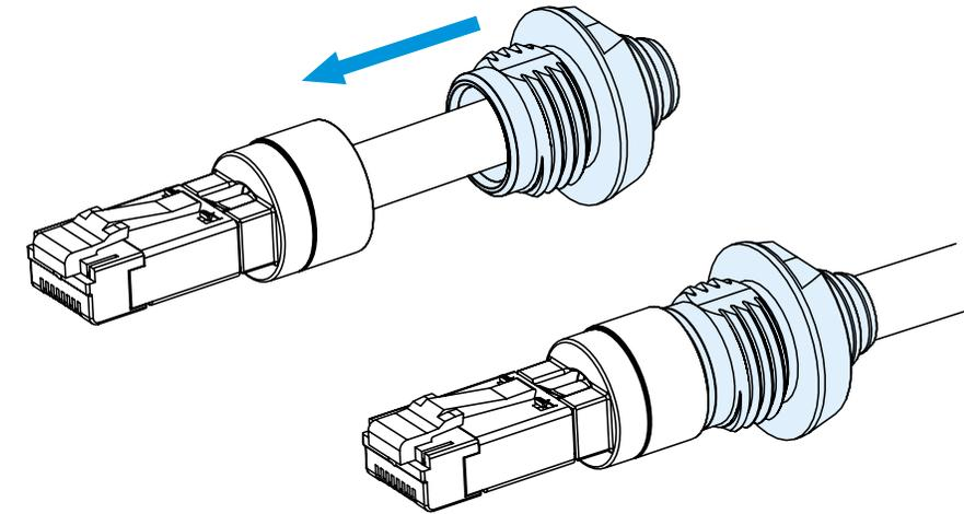
**06** Insert the IP67 cover into the Y-CON-TOOL-40
