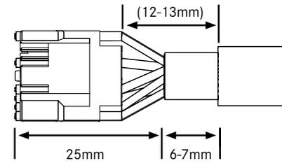
**04** Insert the prepared cable into the plug using the Y-Con Tool-30 until it stops
