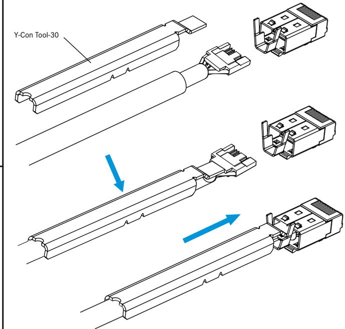
**05** Crimp the plug with the crimping tool as shown
