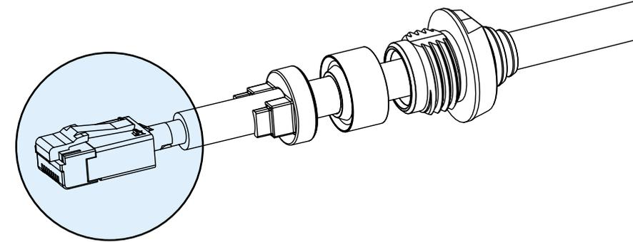
**03** Put the plugstopper into the plug
