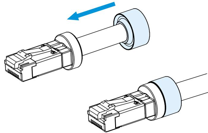
**05** Push the sealscrew to the cablesealing
