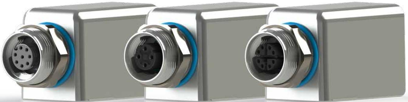
With the new switch cabinet coupler, you can easily switch from an internal RJ45 switch cabinet cabling to an external M12 cabling. Different coding variants (A8, D4 and X coding) ensure adaptation to the required transmission performance and, with the A8, offer the option of transmitting additional power.
