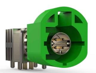
The HSD plug connector system is used for signals like USB or IEEE 1394, for example. For the HSD interface, signal transmission via LVDS (Low Voltage Differential Signaling) is used. This decreases cross-talk between signals and interference from external signals to a minimum. The system is  $100 \Omega$  impedance controlled, so that signal transmission of the highest quality is achieved.
