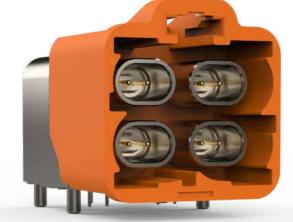
With the Y-HDE series, Yamaichi Electronics offers differential high-speed connectors that provide high-speed data transmission for the automotive sector in the smallest installation space.
