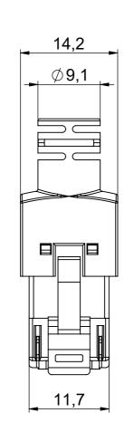
Y-ConKit-12: Plug with power contacts (Y-ConPlug-51/ 8(8)+2) and IP20 strain relief
