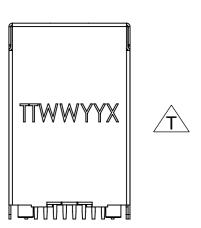
Date code (TypeWeekYear) is printed on the back side of the jack Type: Y-ConJack-51 -> 51
